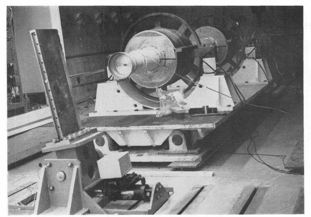
MODEL HOLDER in test cell at Hot Gas Facility is shown in position at left above, with temperature-sensing rod directly in the path of exhaust from Cajun rocket engine positioned in two round
